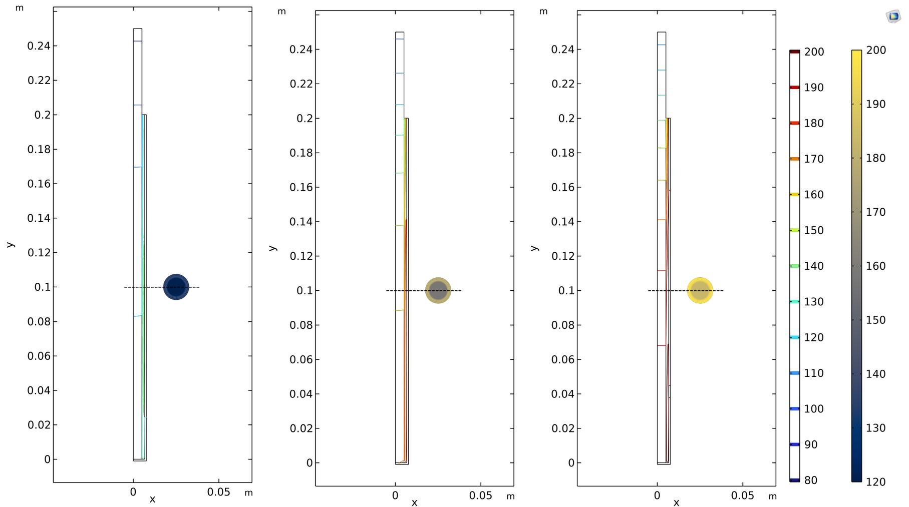
**Figure 5.12:** Single cold finger with cross sectional cut at  $y = 0.1$  m at timesteps  $t = 60$  s (left),  $t = 120$  s (middle) and  $t = 200$  s (right). The plate from the cooling shield has been omitted for displaying purposes.
