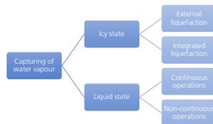
Figure 3: Design option tree for vapour capturing.
