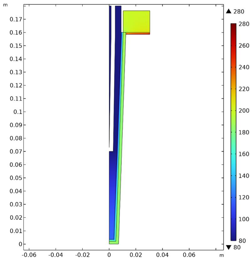
**Figure 5.20:** Ice Collection status with cooling still enabled with 115 W at 495 s.
