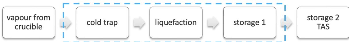
**Figure 5.2:** Scheme for the scope of the water capturing subsystem.
