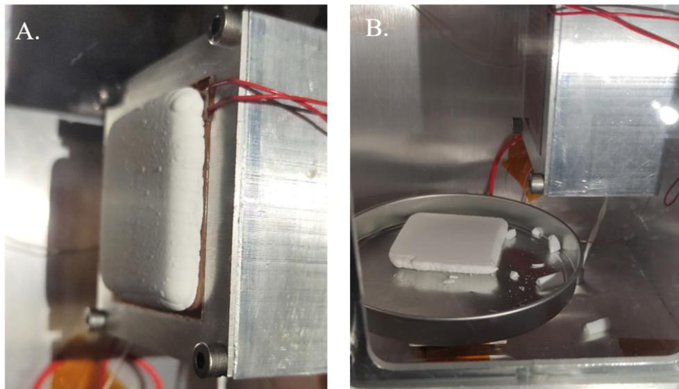
**Figure 1.8:** Maximum ice built-up on the cold plate (A.) and delamination induced by a thin heater (B.). Cold plate dimensions are 40x40 mm. Captured water mass is around 11 g [34].
