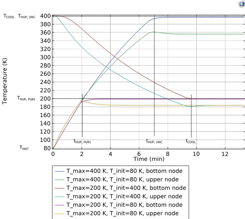
**Figure 5.17:** The three previously discussed modes of operations (Heating up to purification temperature, heating up to delamination temperature and cooling down) in a single plot with an exemplary heat flux power of  $q = 12520 \frac{W}{m^2}$ . Both nodes are represented.
