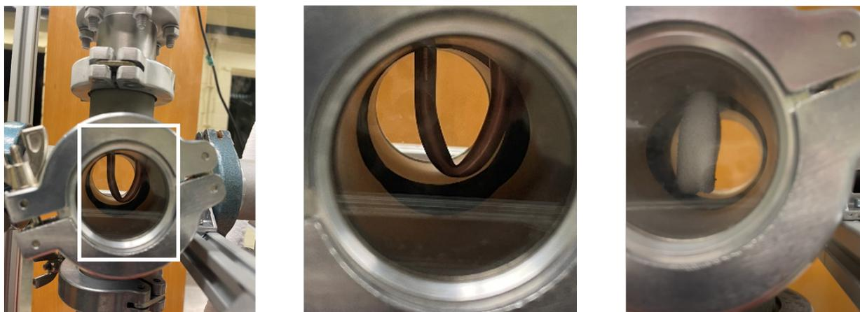
**Figure 4.3:** Close up views of the white rectangle of the cold trap. Middle photo is before the ice deposition which can be seen on the right photo. Glass has a diameter of around 40 mm.
