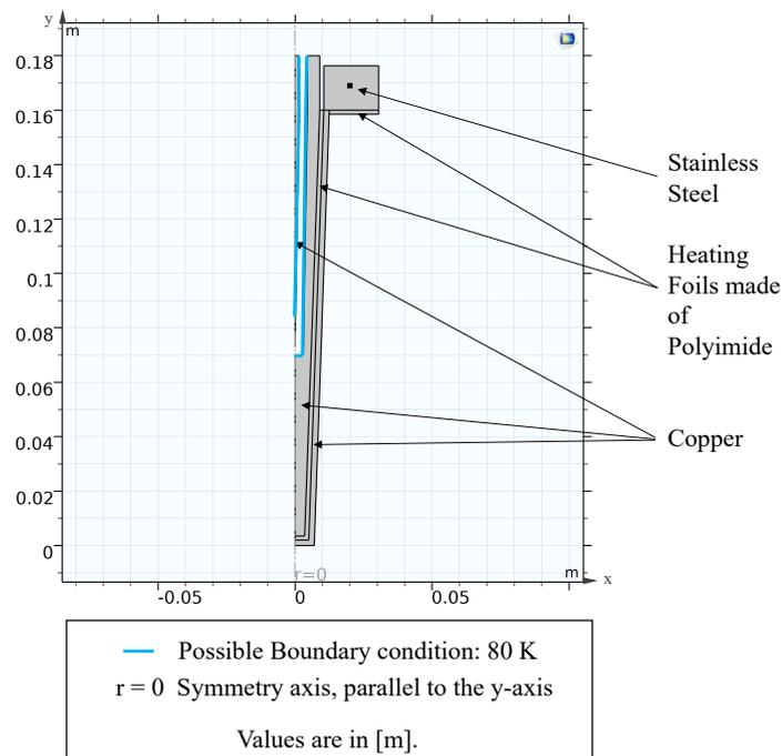
**Figure 5.18:** Sketch of the Geometry, which is rotated.
