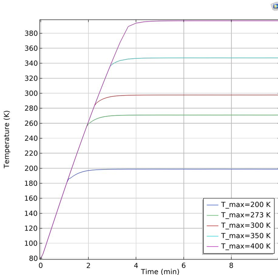
**Figure 5.15:** Heating up further to different ice uncoupling temperatures with  $q = 20000 \frac{W}{m^2}$
