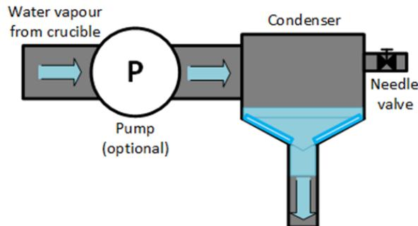
**Figure 3.7:** Schematic for a condenser. Figure courtesy of [43].
