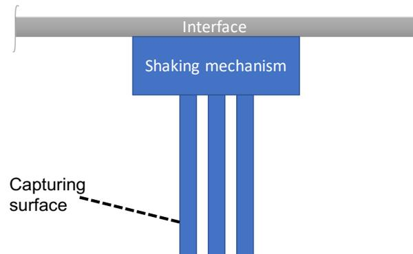
**Figure 3.9:** Schematic for a centralised shaking mechanism. Rods are only an example of a possible collection surface geometry.
