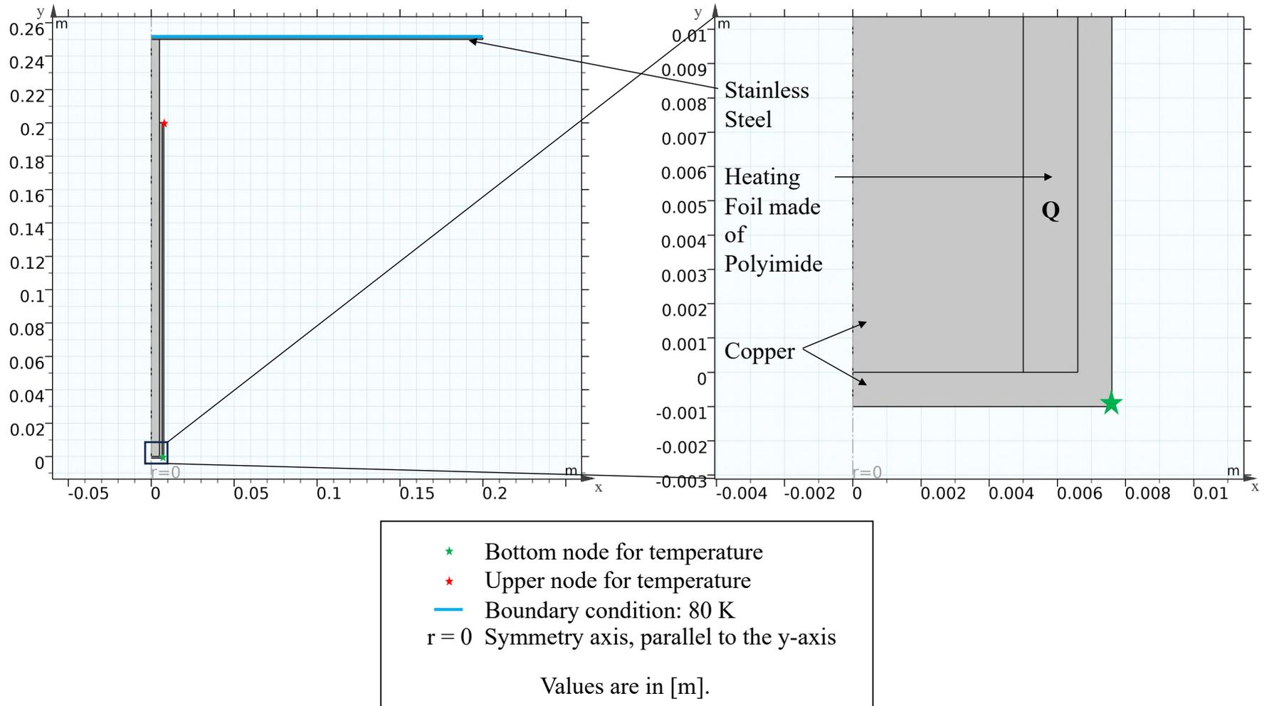
**Figure 5.10:** Geometry of the Simulation Model. Ambient environment temperature is set to 80 K. Heat  $Q$  is modelled as a volume heat source to the heating foil.
