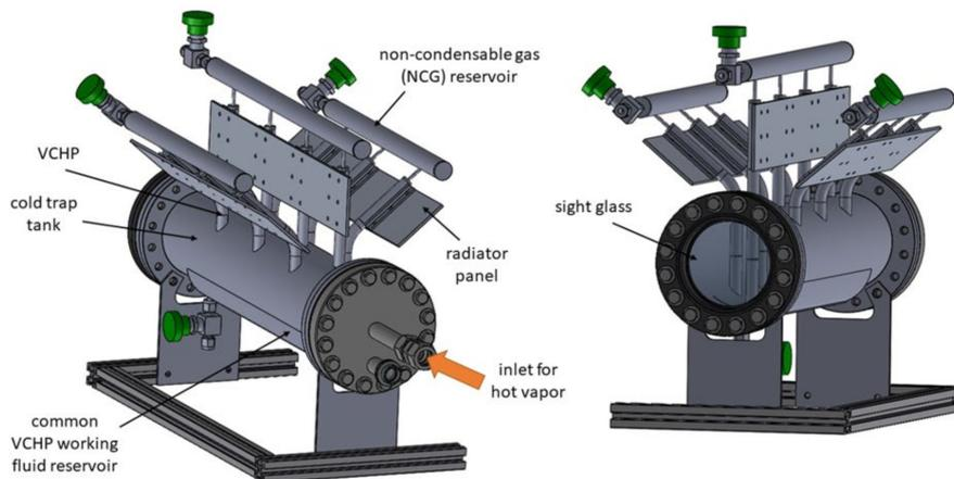
**Figure 1.10:** Next Iteration of the Cold Trap Chamber [30].
