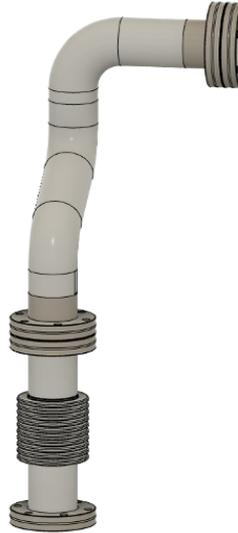
**Figure 5.4:** Piping from the WES to WCS with flex tube on the bottom section. [48] [50]
