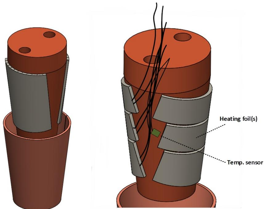
**Figure 4.8:** CAD-Schematic of the cold finger with channels, attached foils and sensor and shell below. Figure courtesy of [43].
