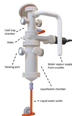
Figure 5: Model of the cold trap and liquefaction.
