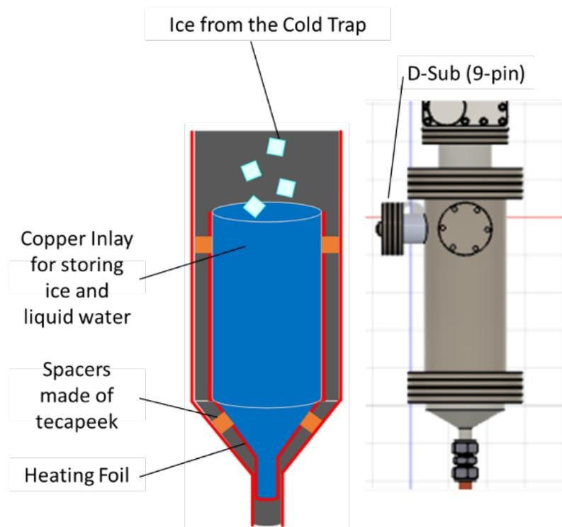
**Figure 5.8:** Liquefaction Sketch (left) and outside CAD view (right). Courtesy CAD of [48]
