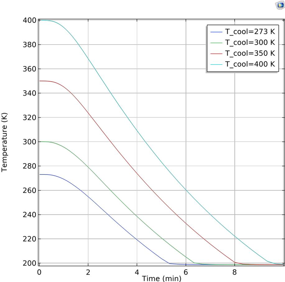
**Figure 5.16:** Temperature over time with different initial temperature of the copper rod, heating foil and copper shell.
