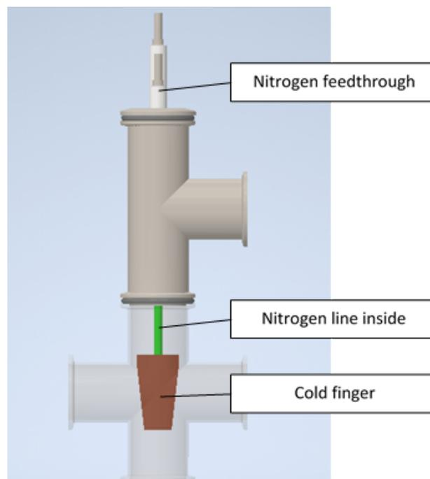
**Figure 4.6:** Scheme for the uncoupling experiment. Figure courtesy of [43].
