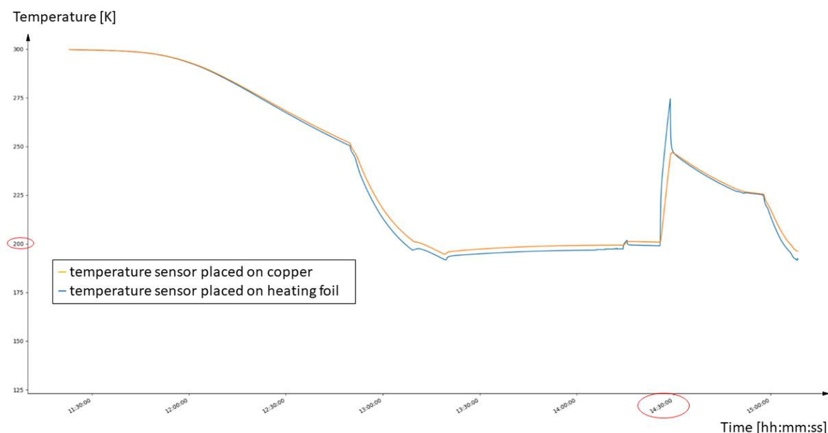
**Figure 4.5:** Temperature graph. Maintaining temperature at 200 K and small delamination peek at 14:30:00 h (both encircled). Based on [41] and [48].
