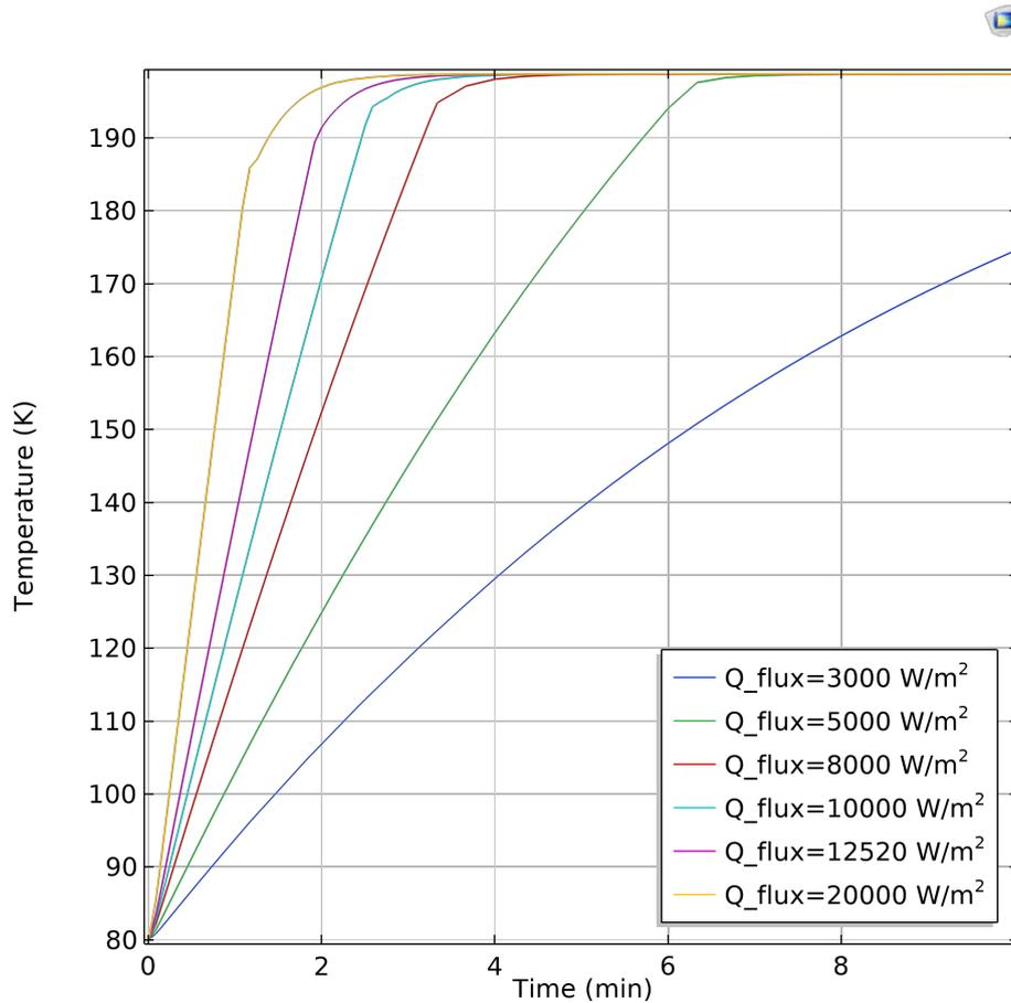
**Figure 5.11:** Temperature of the bottom node over time for different heat flux densities  $q$  ( $Q_{flux}$ ).
