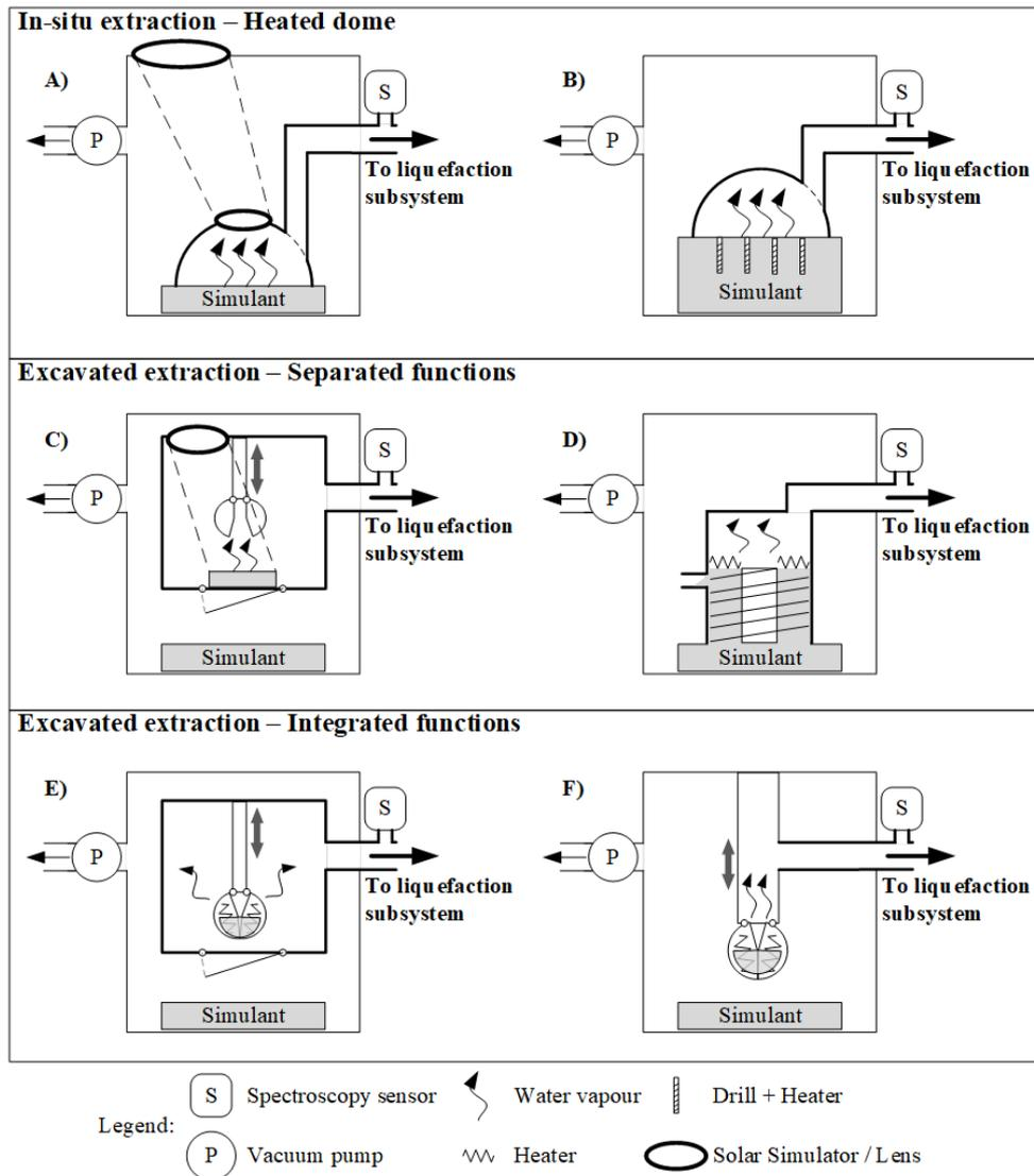
**Figure 1.6:** Schematic overview of possible water extraction methods [28].
