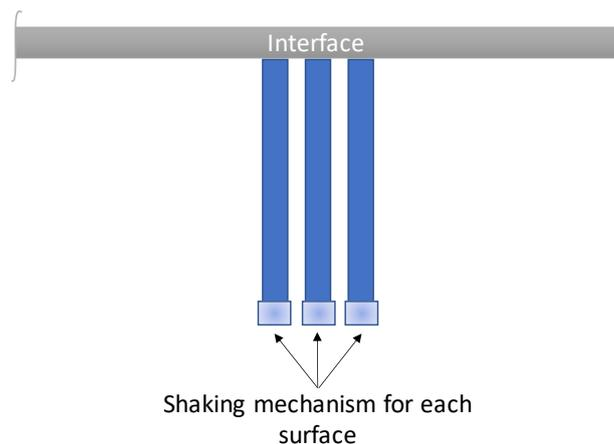
**Figure 3.10:** Schematic for individualised shaking mechanisms. Rods are only an example of a possible collection surface geometry.
