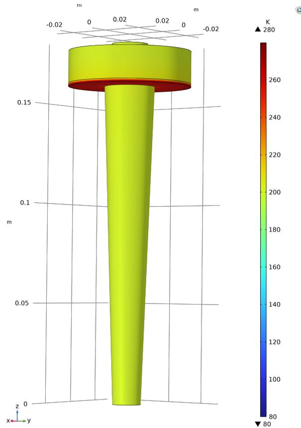
**Figure 5.19:** 3D-view after the revolution. Foil beneath the shell has a power of 115.2 W, compare table 5.9. 378 s were needed to reach this state.
