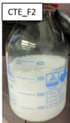
**Figure 1.7:** Post-test cold trap photos with water ice built-up between 11.4 and 21.2 g. Bottle height is 17.6 cm [33].
