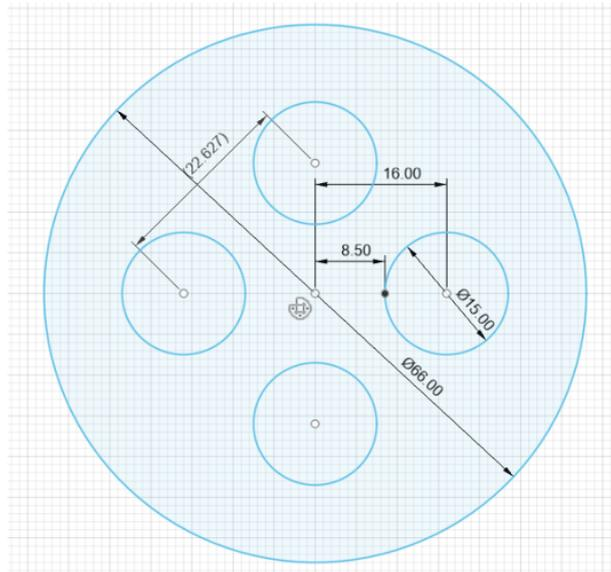
**Figure 5.6:** Arrangement of the cold fingers inside the cold trap chamber.
