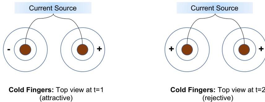
**Figure 3.11:** Concept for vibration induced by magnetic fields on two metal rods. (Top view)
