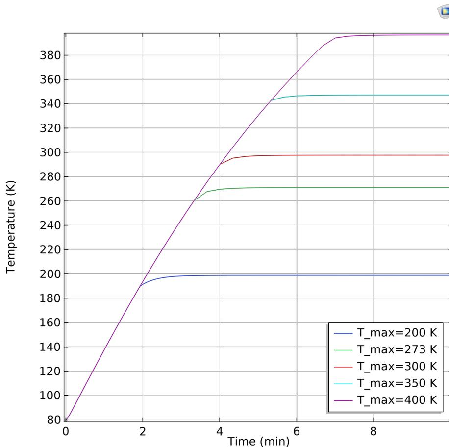
**Figure 5.14:** Heating up further to different ice uncoupling temperatures with  $q = 12520 \frac{W}{m^2}$ .
