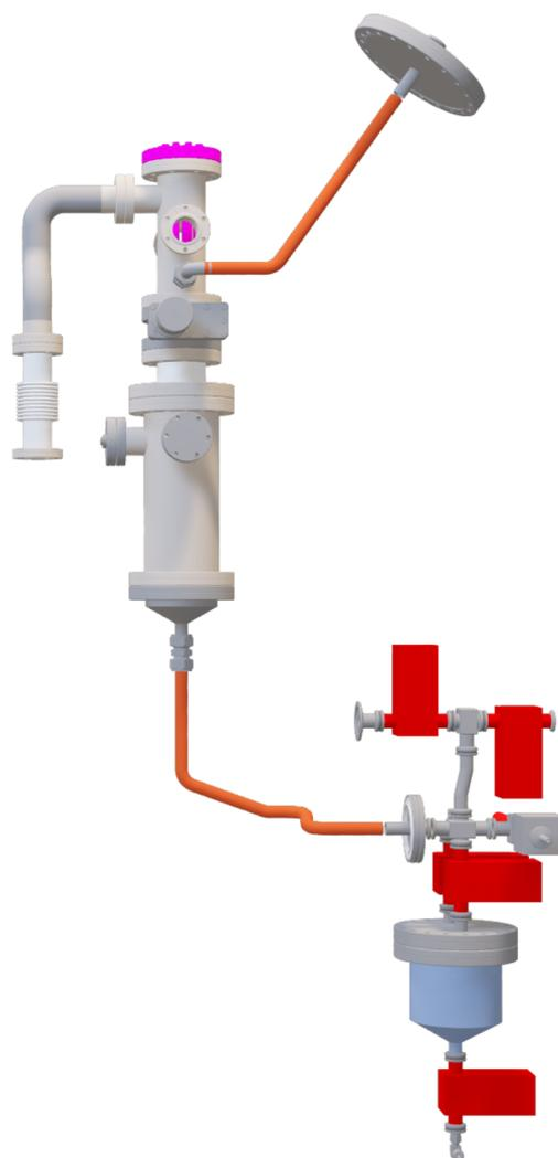
**Figure 5.3:** CAD-View of the capturing subsystem with Storage 1. Red boxes are valves. Figure courtesy of [48] and [50].
