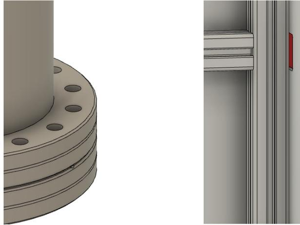
**Figure 5.9:** Flange (left) with holes for M8-screws and aluminium frame (right). CAD Courtesy of [48].
