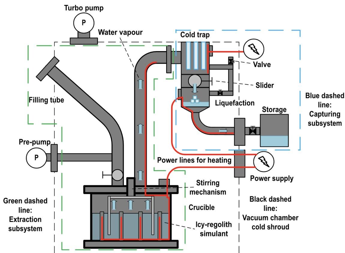
**Figure 5.1:** Sketch of the extraction and capturing system inside the TVAC. Figure courtesy of [43].
