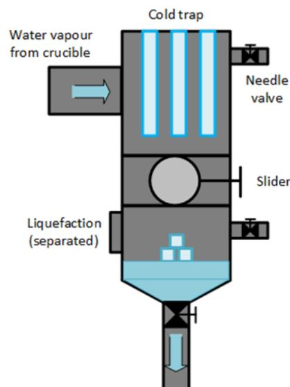
**Figure 3.5:** Schematic for a cold trap with external liquefaction. Figure courtesy of [43].
