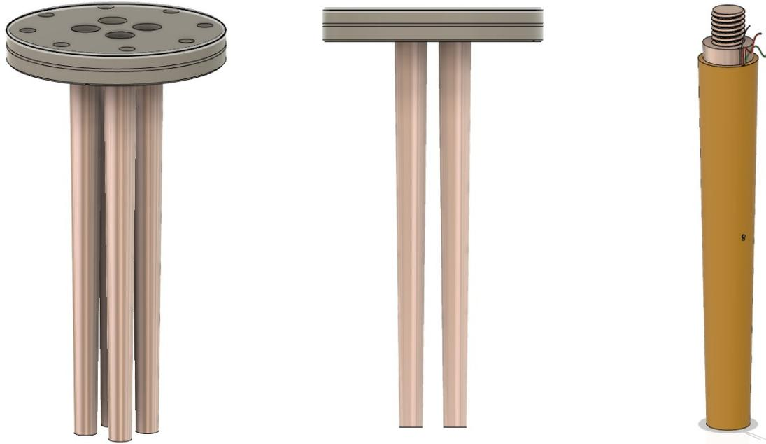
**Figure 5.5:** Cold trap top flange with attached cold finger shells and a cold finger for the insertion in the shell with wrapped heating foil and temperature sensor in the middle (thread outdated).
