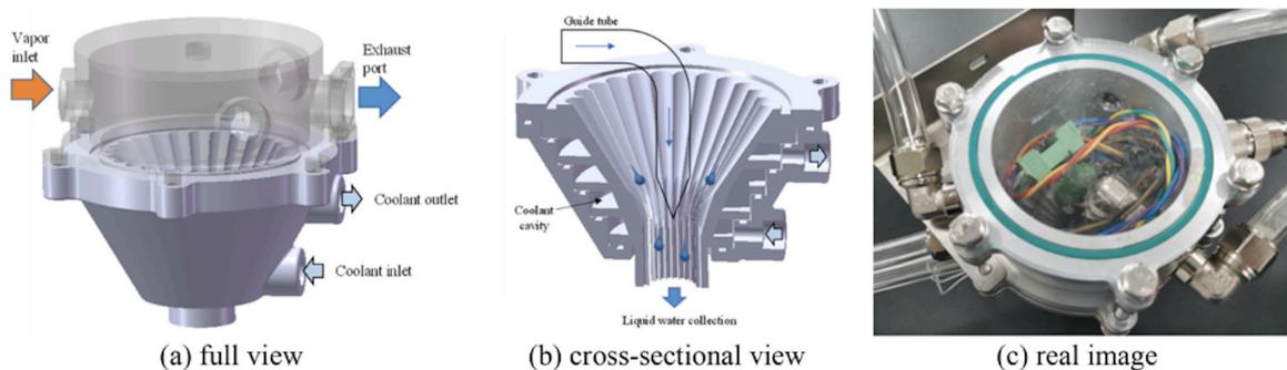
**Figure 1.11:** Condenser in CAD and in experimental setup. Captured water between 16 to 51 g [31].
