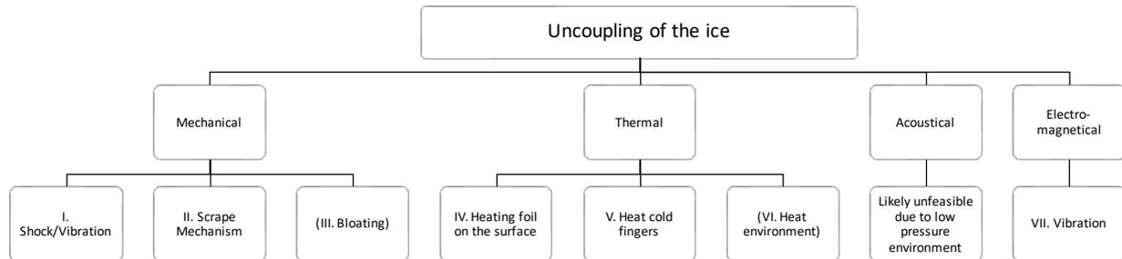
**Figure 3.8:** Design Option Tree for uncoupling of the ice from a cold surface.
