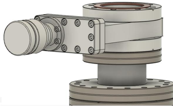
**Figure 5.7:** CAD-view of the slider and extension flange. [41] [48]
