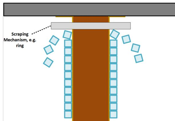
**Figure 3.12:** Scraping Mechanism. Brown is a cut of a collection surface.
