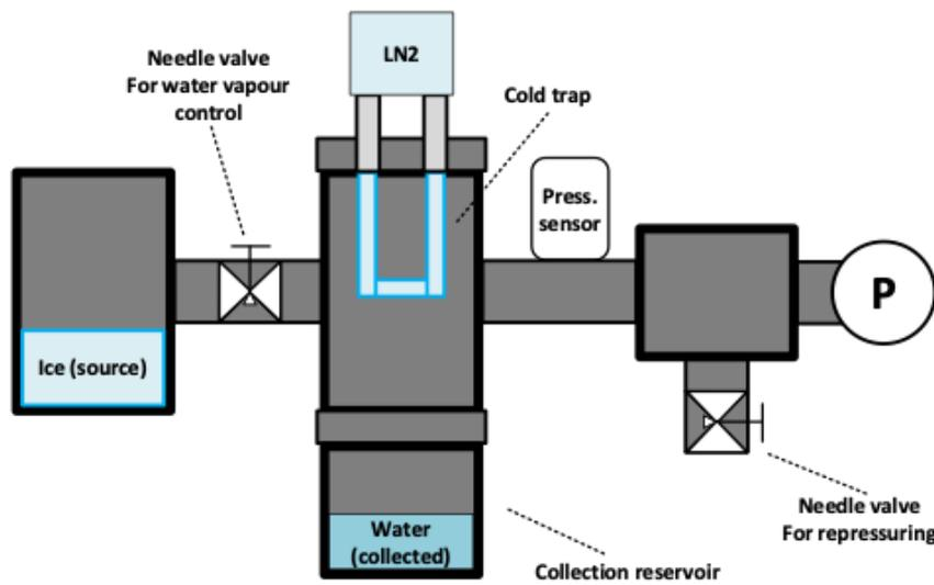
Figure 4.1: Schematic of pre-experiment I setup. Figure courtesy of [43].
