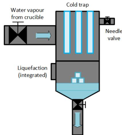
**Figure 3.6:** Schematic for a cold trap with internal liquefaction. Figure courtesy of [43].
