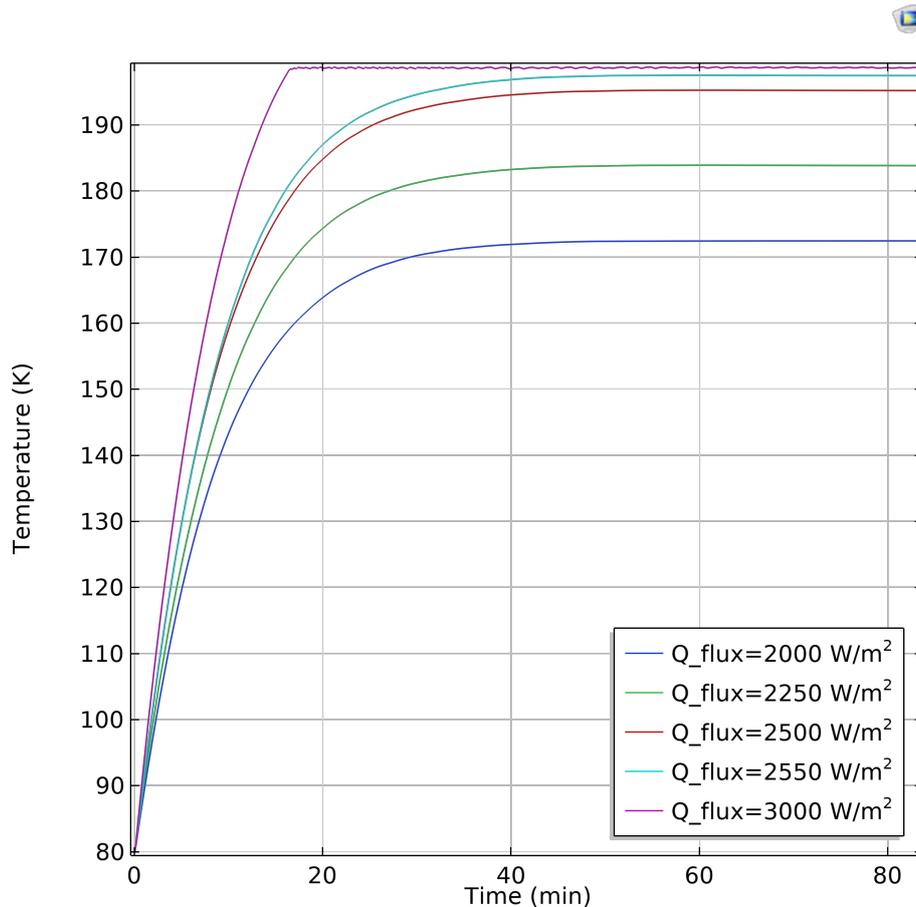
**Figure 5.13:** Bottom node temperature over time with too low heat flux densities  $q$ . Chatter on the purple graph is because of the on/off of the heat source to keep the temperature at 200 K.
