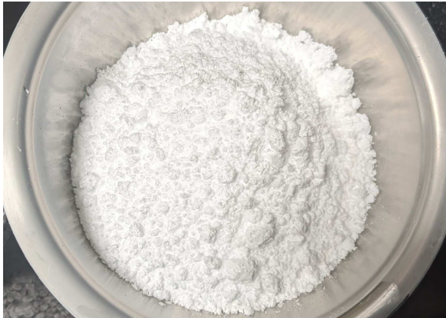
Figure 3.5.: Desiccated water ice particles in a metal bowl. In the sample, numerous agglomerates of up to a few millimeters in size are visible. The diameter of the bowl is approximately 125 mm.
