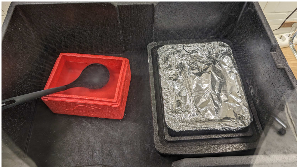
Figure 3.7.: Setup for the cool-down process of regolith simulant samples. Liquid nitrogen cools the metal sample container (covered with aluminium foil, approx. 20 cm wide) and provides a dry atmosphere. The entire setup is located in a glove box to further limit the influence of humidity.
