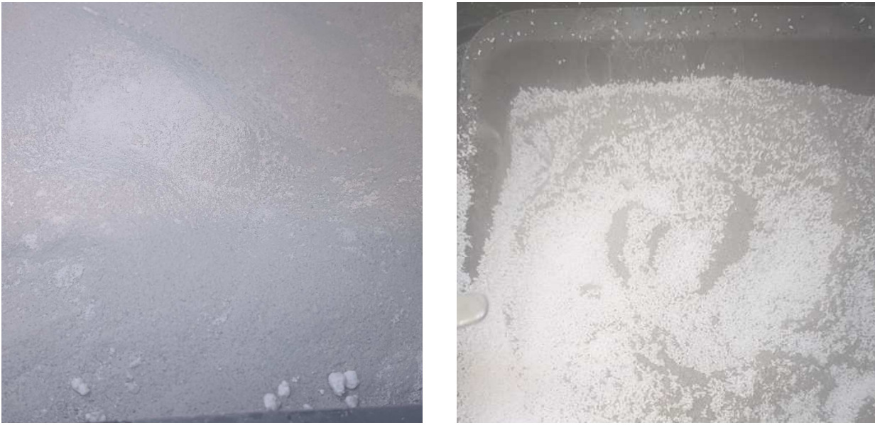
Figure 3.11.: Desiccated ice particles sieved onto a dry regolith simulant sample with a sieve opening of 250 \mu\text{m} (left) and 1000 \mu\text{m} (right). The sieved ice particles can be distributed evenly and can be made much smaller than the unsieved agglomerates (left bottom).
