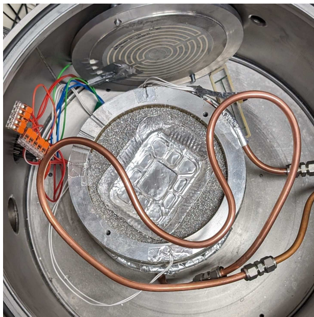
Figure 4.2.: Sample holder inside of the TVAC. The copper pipes of the cooling system run along and above the sample holder. There are three heating foils in total, one of which is visible on the lid next to the sample holder. The other two are attached to the inner bottom (not visible here) and inner side wall of the sample holder. A Pt-1000 sensor is located inside the aluminium wall.
