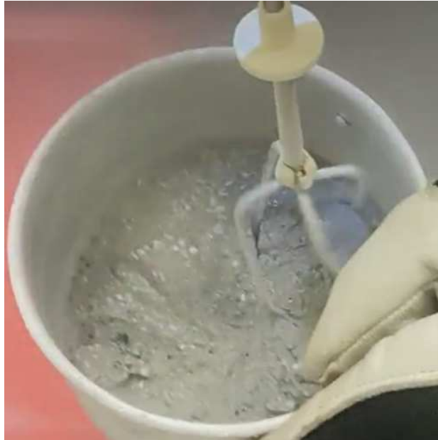
Figure 3.9.: Whisking of an icy regolith simulant with agglomerates with a power tool has no significant effect on the number of agglomerates. The largest ones seem to break into smaller ones of approximately 1 mm in size.
