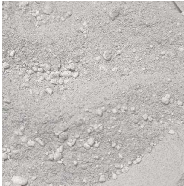
Figure 3.8.: Agglomerates in an icy regolith simulant sample mixed with desiccated ice particles and without liquid nitrogen. The largest agglomerates visible here are approximately 4 mm in size.
