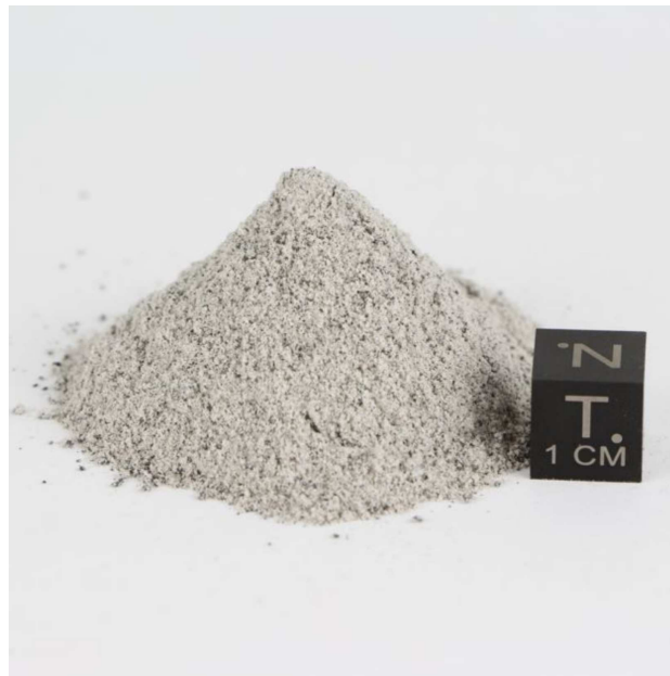
Figure 3.2.: A small pile of LHS-1 appearing as a fine gray powder with some darker grains [23].
