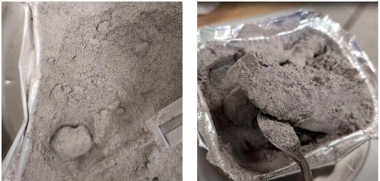
Figure 6.42.: Cemented chunks in Icy LHS-1 2 (left) and Icy LHS-1 3 (right) that were removed from the TVAC before complete desiccation. The visible ice-regolith chunks did not exhibit much mechanical strength and could be easily broken with a pointy metal tool but are clear evidence of a cementation process.
