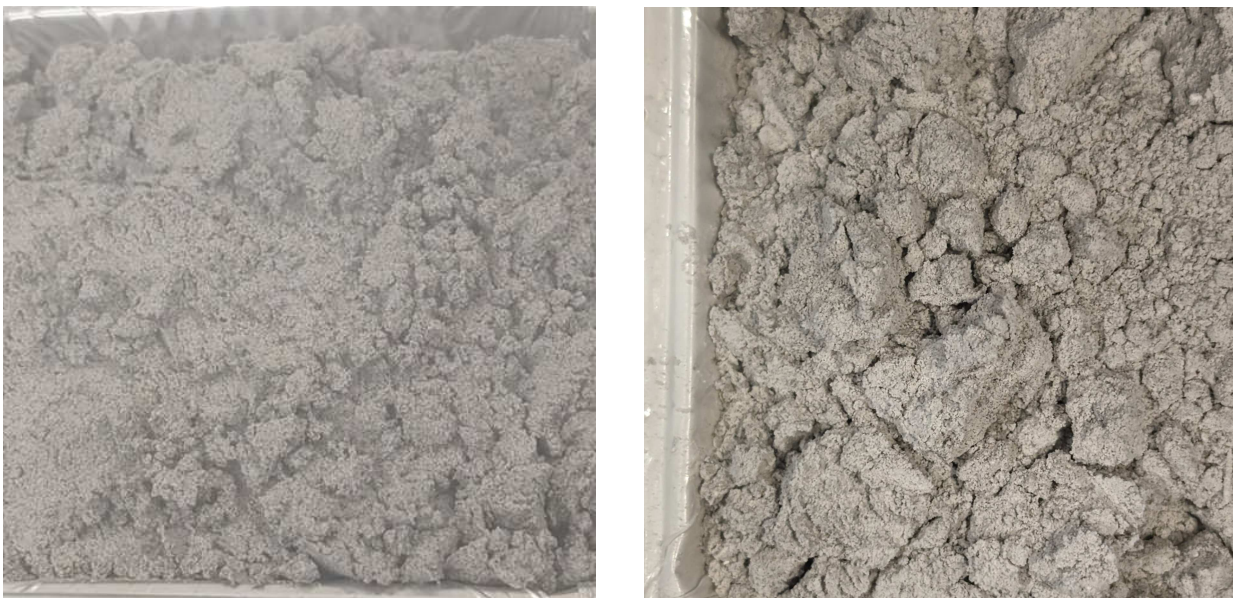
Figure 3.13.: Microgranular icy regolith simulant samples with an ice content of 2.9 wt % (left) and 7.7 wt % (right) after most of the liquid nitrogen evaporated. No major trace of ice agglomeration is evident in those approximately 7 cm and 5 cm wide frames, indicating a mostly homogeneous mixture.
