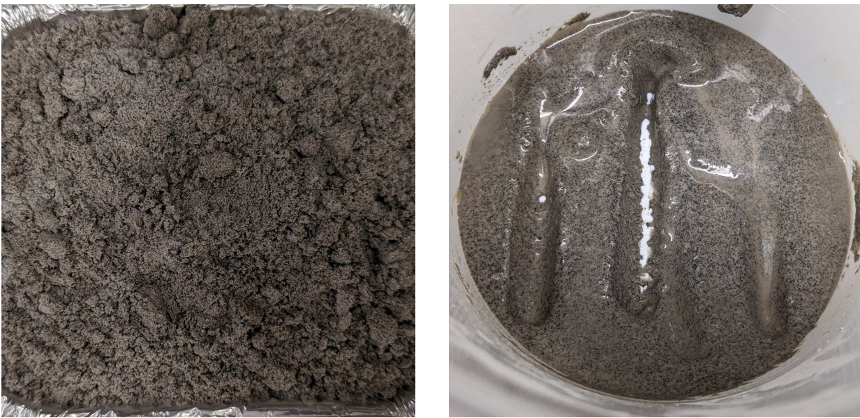
Figure 3.14.: Mudpie simulant prepared by mixing the regolith simulant with demineralized water with a water content of 2.9 wt % (left) and 23.1 wt % (right) resembling wet sand and mud respectively. The additional water visible on the right side of the image is a result of the sample being over-saturated with water. The samples shown here are not frozen yet.
