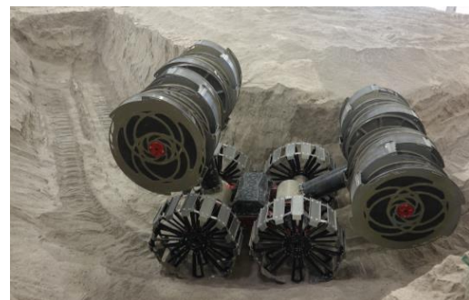
Figure 2-7: Possible combination for crucible heating with a heating chamber setup (left) (Reiss 2018b) and a bucket drum excavator to deliver the regolith (right) (modified from Just et al. (2020))
