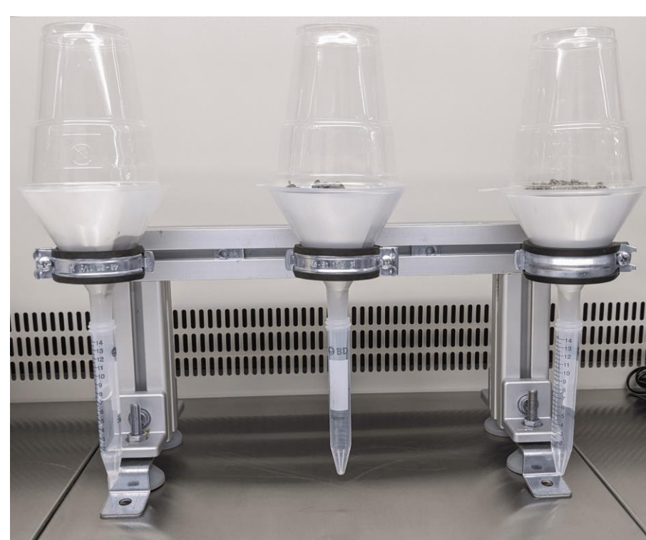
Figure 2: Test-setup water in lunar regolith (saturation occurs at around 16%).
