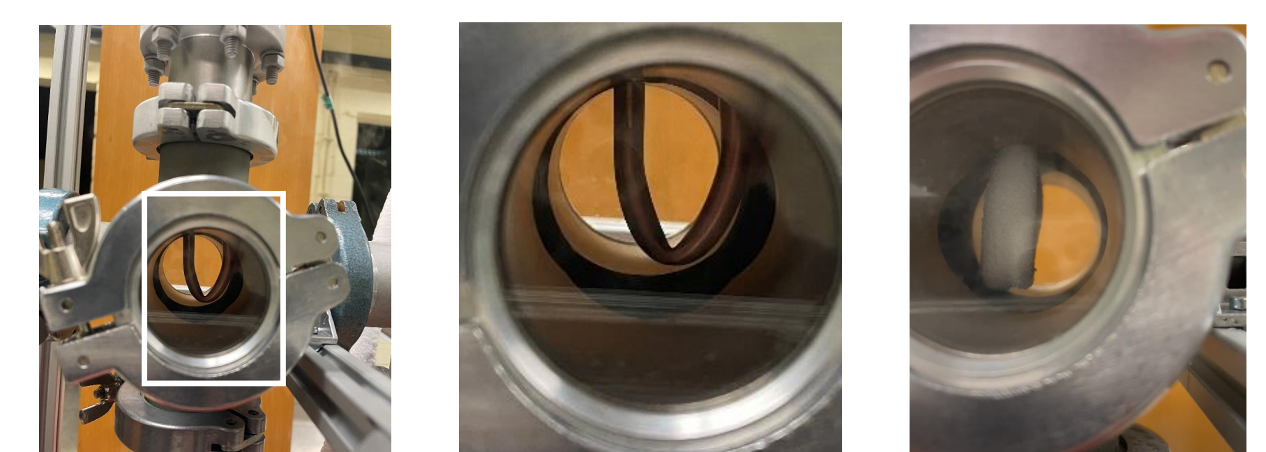
Figure 7: Cold trap without ice (left) and with ice (right).
